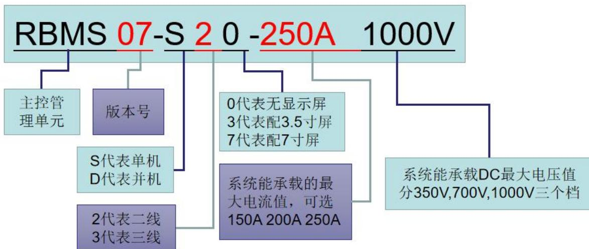
Example: RBMS07 D37-250A 700V represents that the GCE series BMS supports parallel, three-wire system, with a 7-inch display, and supports a maximum current of 250A and a voltage of 700V.
